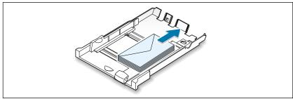
5. Slide both paper adjusters to fit against the paper's edges. Ensure the paper line flat in the tray and fits under the tab of the paper-length adjuster.
